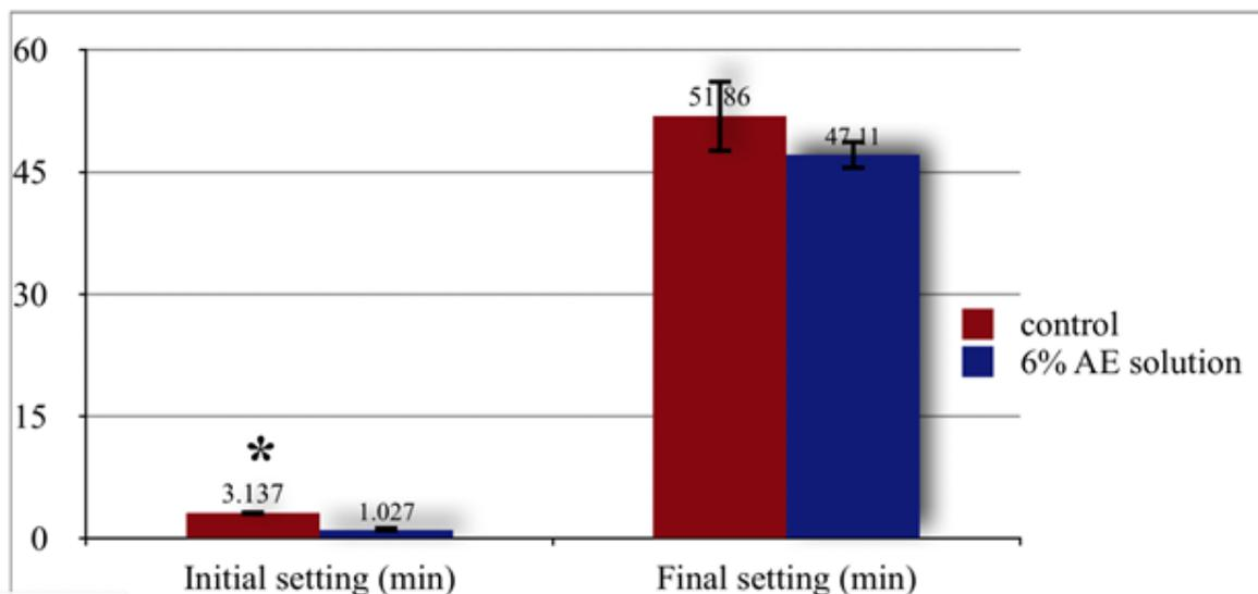
Figure 3. Comparison of setting time of plaster mixed with with tap water and one with tested solution (\*  $p < 0.05$ )
