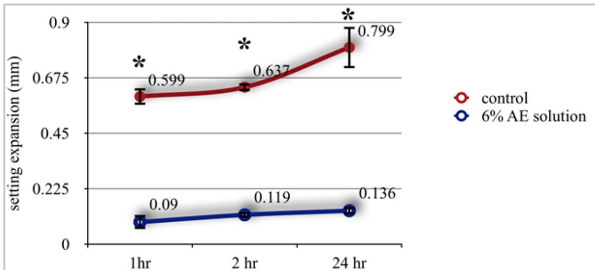
Figure 2. Comparison of setting expansion of plaster mixed with tap water and one with tested solution (\*  $p < 0.05$ )
