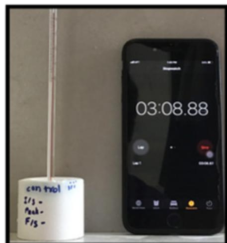
Figure 1. Experimental design for measuring plaster expansion (upper panel) and measurement of setting time through temperature change recording (lower panel)
